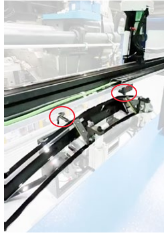
Work piece is locked in jig for laser cutting.
