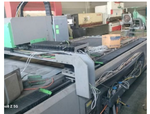
Retrofit old cable & wire
