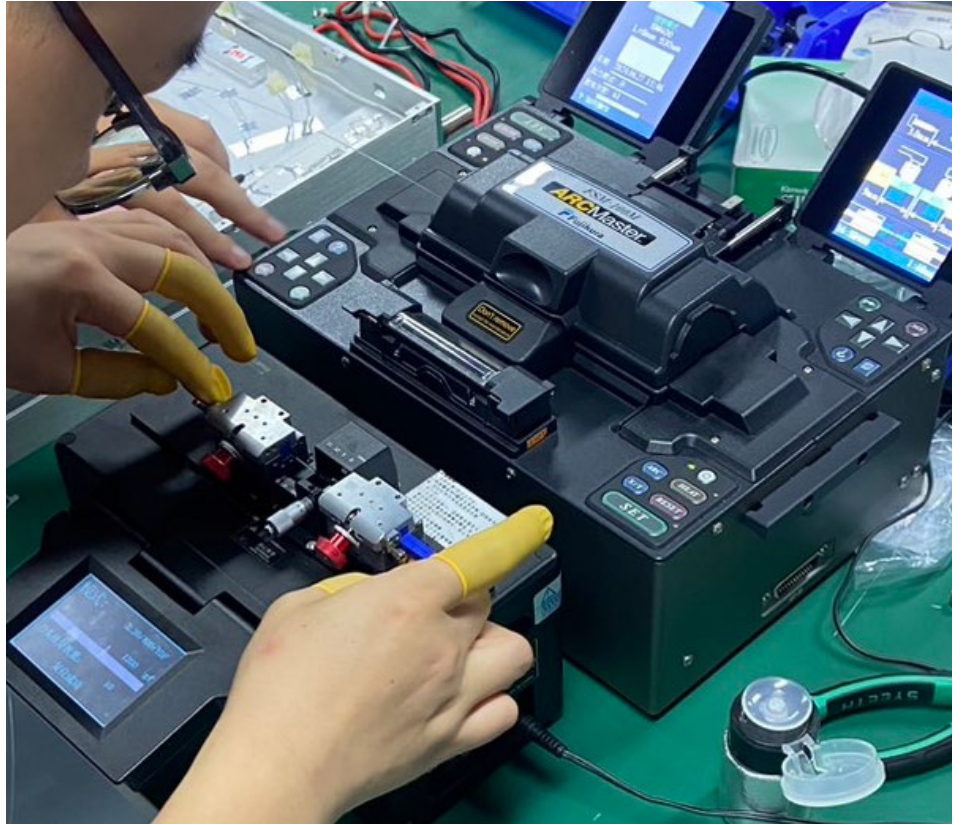
Fiber alignment and welding
